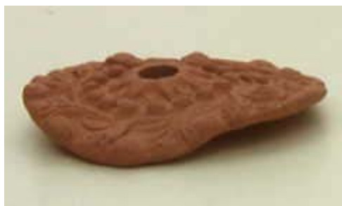
Sample of a heat dried piece. Very fine stress cracks developed during drying. The sample was chip carved to see if it had any affect on the opening of the cracks during sintering.
