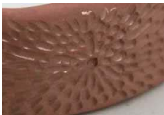
Sample of a heat dried piece. Very fine stress cracks developed during drying. The sample was chip carved to see if it had any affect on the opening of the cracks during sintering.
