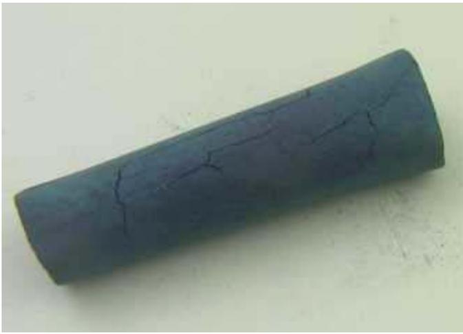
*Example of a heat dried piece that developed stress cracks. The photo shows the sample after firing. Before firing, the sample had only hairline cracks barely visible on the surface*
