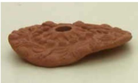
The internal stress of uneven drying also causes warping of the item being dried. Thin pieces are more susceptible to warping, but all BRONZclay pieces can warp when dried un-evenly.
