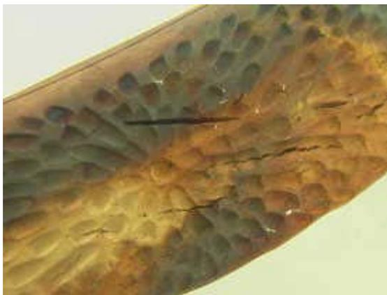
*The hairline cracks observed before firing have opened up during sintering. Chip carving the surface had no effect in deterring the cracks.*
