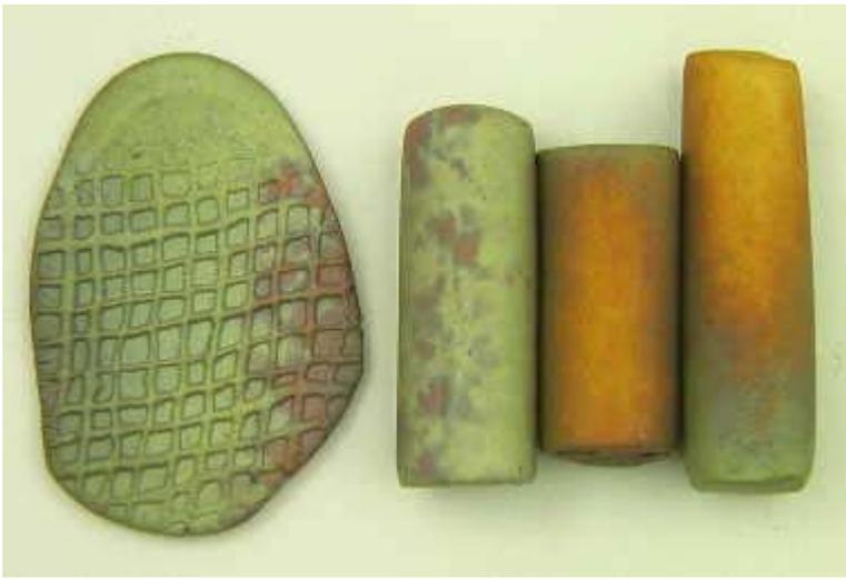
*The 3 rods at the right were fired completely wet. The slab on the left was frozen before firing.*
