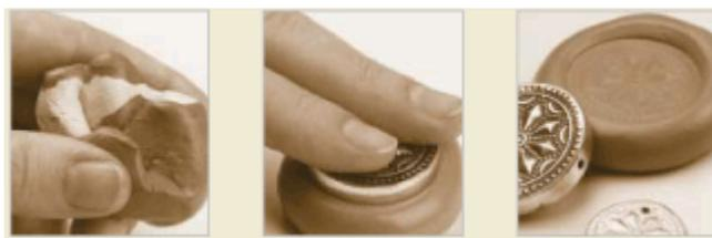
Using 2 Part Silicon Mould to make a mould
